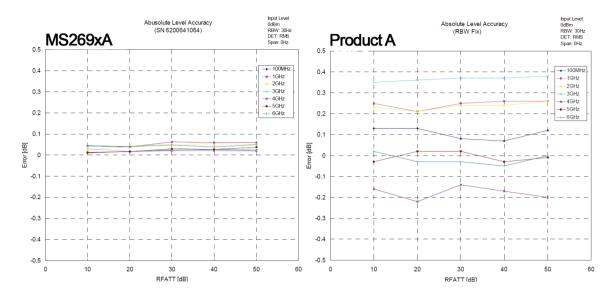
In figure 2 we can see the difference between the Anritsu MS2830A absolute level accuracy versus a conventional Spectrum Analyzer from another supplier. The impact of the Anritsu calibration circuits can be seen with two effects.
