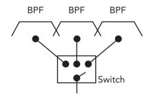
The filter bank technique uses a set of Band Pass Filters (BPF), and these each have typically a bandwidth of 400 MHz. A switch is then used to select a matrix of different BPF to give the required high band selectivity. These filters are implemented using printed circuit techniques, to give low cost, low power consumption, and high stability. The stability comes from there being no tuneable or variable circuits involved.
