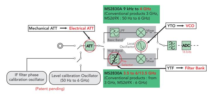
It is seen in figure 1 that the calibration signal is swept across the frequency range 50 Hz to 6 GHz in the MS2690A series (and to 4 GHz in the MS2830A series), this validating the compensation across this whole range, and in addition this compensation circuit includes the input level attenuator as well as the whole receiver chain. This level accuracy is maintained across the whole 6 GHz frequency range and with the full range of input attenuator settings (up to 4 GHz in the case of MS2830A).
