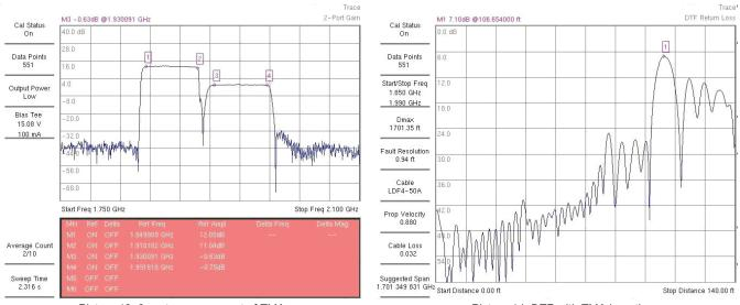
Picture 13: 2-port measurement of TMA
