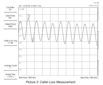
Increasing the RF frequency and the length of the cable will increase the insertion loss. Cables with larger diameter have less insertion loss and better power handling capabilities than cables with smaller diameter.
