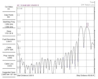
Picture 12: DTF PCS antenna with fault
