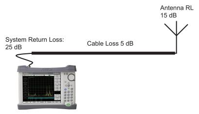
Picture 4: System Return Loss setup
